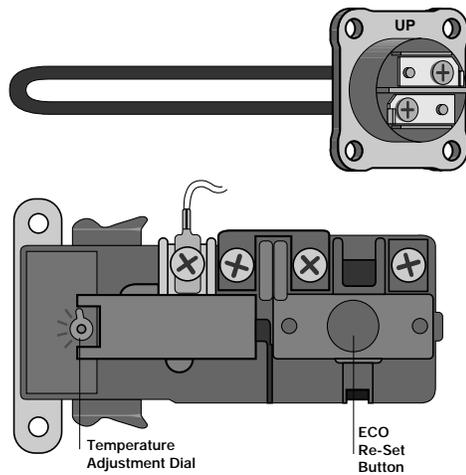
Early model water heaters with 110 VAC heating capacity used a bolt-on heating element and a one piece thermostat/E.C.O..
