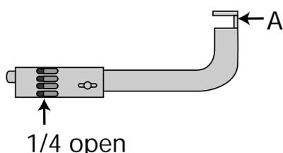
At the end of the burner tube there is a dime-shaped deflector disk. This disk spreads the flame out for proper heat distribution. Align the flame spreader (A) so that it is parallel to the end of the tube and positioned in the center of the end of the tube. If the flame spreader is out of position, it could divert the gas away from the spark and cause intermittent ignition.
