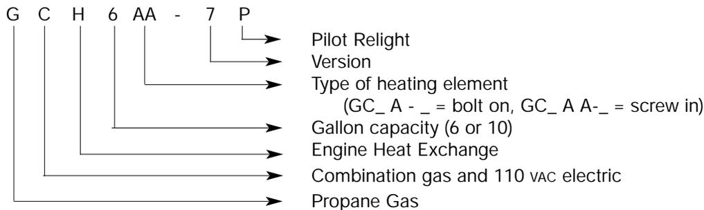
**NOTE:** When replacing the element on a combination gas/110 VAC unit, always check the back of the heater for the type of element it has. It will either be a bolt-on or screw-in element. They are no interchangeable.
