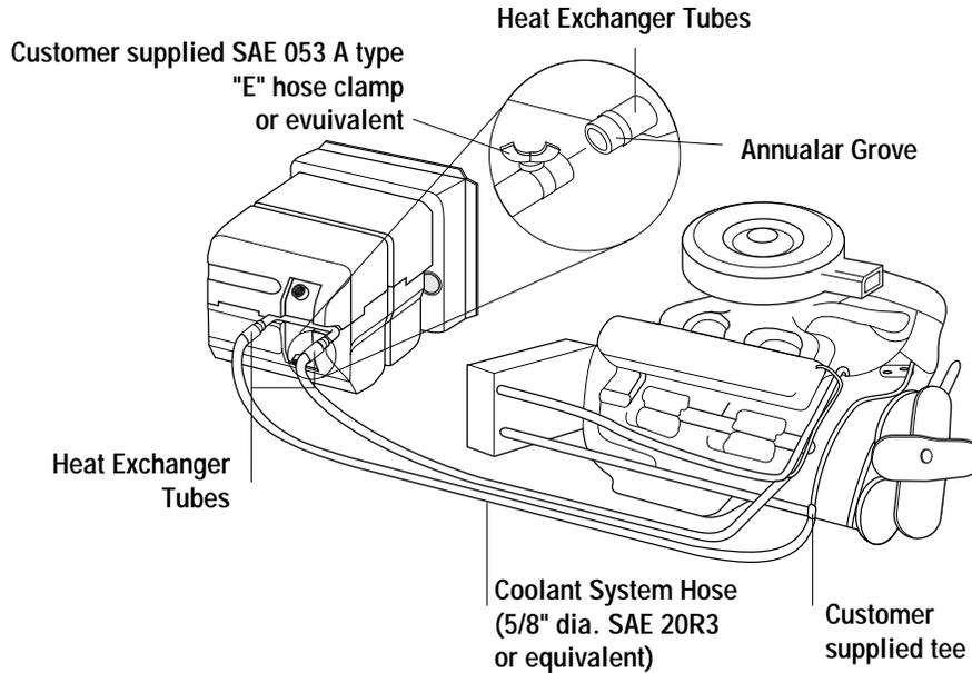
The engine heat exchange system allows a motor home to heat the water while traveling. This convenient option allows you to arrive at your destination with hot water. Operating a pilot or electronic water heater on gas while in transit is a dangerous practice.
