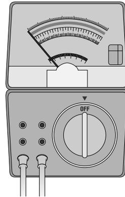
**Circuit Board Tester** - The tester is capable of testing any of the circuit boards (Fenwal and Channel models) that we have used on our water heaters. It is a simple table top device that will diagnose the following items on a circuit board: power circuit, sense circuit, spark generation and the lock-out mode. For use on circuit boards with a flying lead connection, splice a wire into the black wire of the tester harness with a 1/4" male terminal on the free end.
