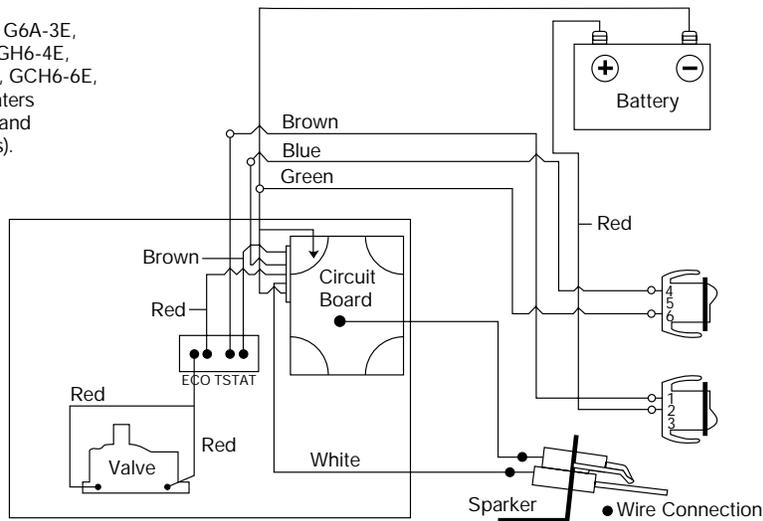
Wiring Schematic G6A-7E, GH6-7E,
