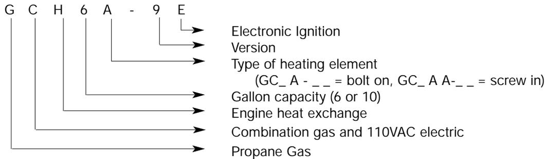
**NOTE:** When replacing the element on a combination gas/110 VAC unit, always check the back of the heater for the type of element it has. It will either be a bolt-on or screw-in element. They are not interchangeable.
